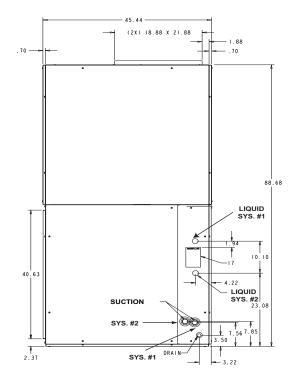
FIGURE 22 - LB480 PIPING CONNECTIONS
